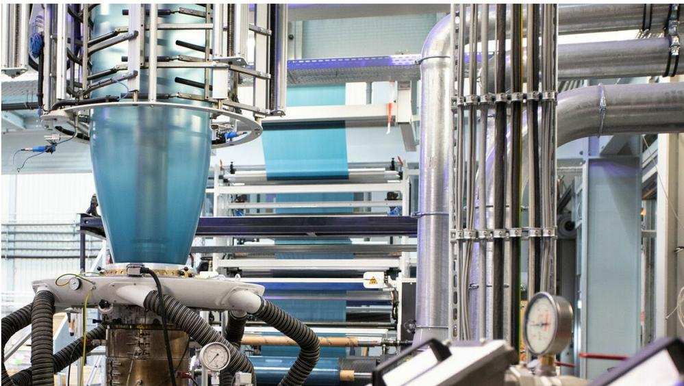
Thanks to the twin-screw and degassing unit, the EVO Fusion extruder can also process low-quality recycle to blown film safely.
