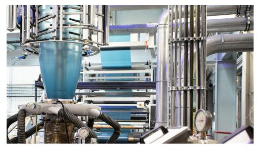
Thanks to the twin-screw and degassing unit, the EVO Fusion extruder can also process low-quality recyclate to blown film safely.
