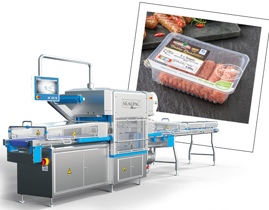
Picture 1: Packaging of fresh meat on a SEALPAC Amax traysealer.
