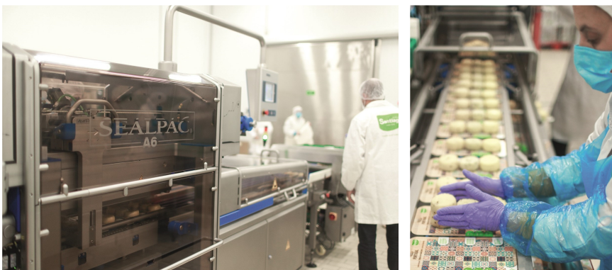
Picture 8a / 8b. The SEALPAC A6 traysealer produces striking FlatSkin® packs based on product carriers with typical Portuguese tile prints.
