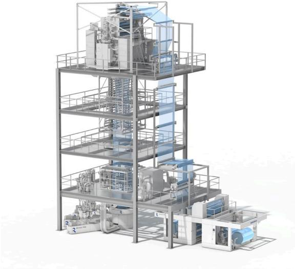
**Reifenhäuser EVO Ultra Stretch: The position of the stretching unit directly in the haul-off of the blown film line is patented and is a unique selling point on the market.**
