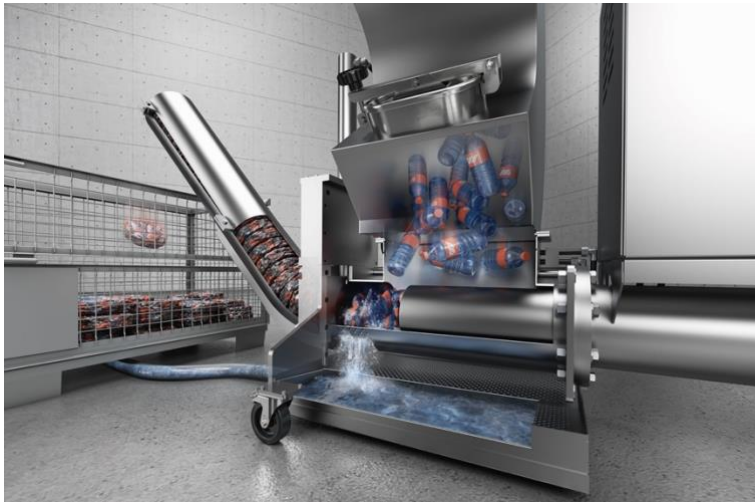
Picture 1: Drainage of PET bottles with a PUEHLER E. series press
