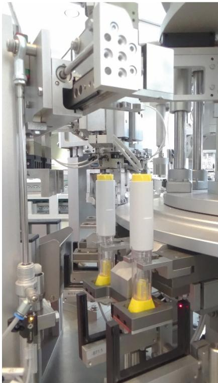
Assembly systems for pen and auto-injectors are one of R+E Automation's strengths.
