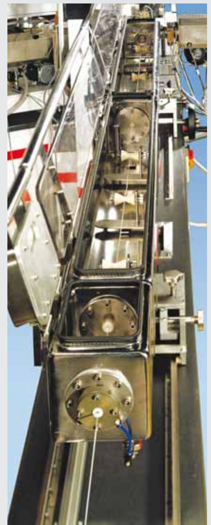
View of an open calibration tank
