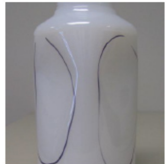
Panel Sink 1: Black marks indicate the extent to which the side panels on this bottle have shrunk.
