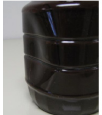
Panel sink 3 The design of this bottle did not provide enough strength to resist panel sink.
