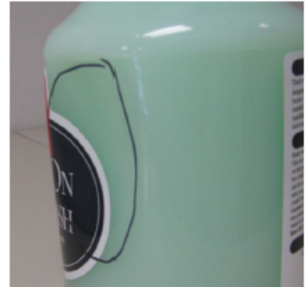
Panel sink 2 The panels on this bottle have begun to sink, but have not yet affected the adhesion of the label.
