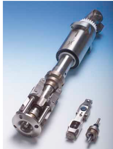
The removed capping head, a thread roller arm and the plunger
