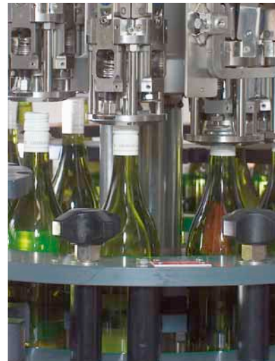
Rolling on of caps onto bottles
