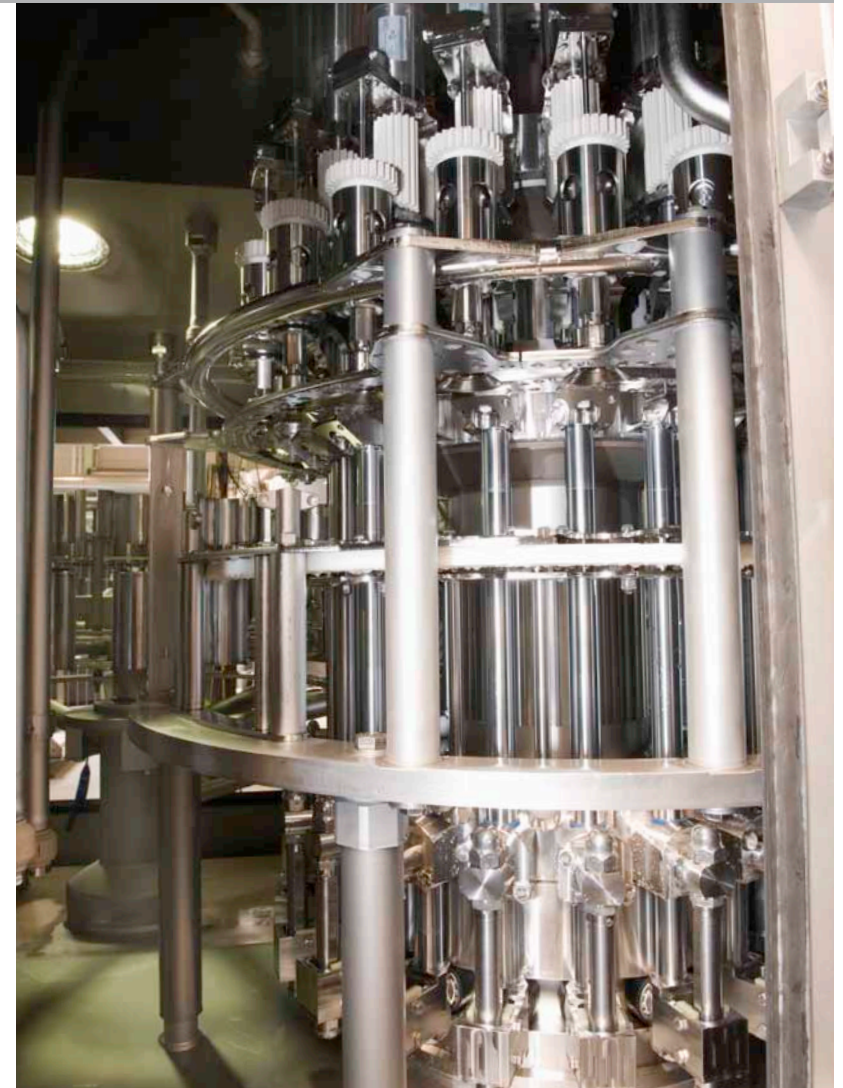
Control cam below the bottle neck finish
